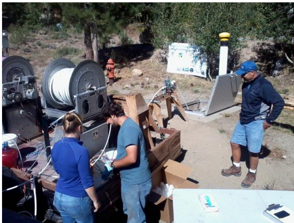
Above: Well-profiling rig at sampling well.
